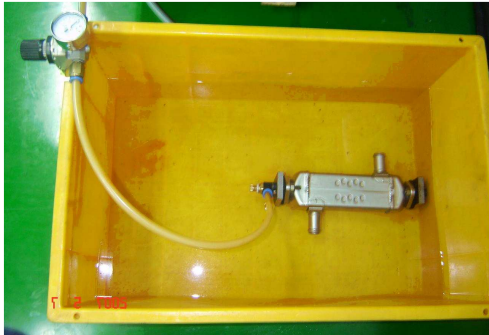
(b) Leakage test
