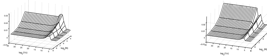
FIGURE 3. Surface plots of the maximum pointwise errors as a function of N and \varepsilon for the solution generated by methods HDS-I and HDS-II of the Example 1.
