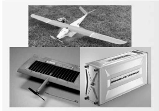
Fig. 6 Example of fuel cell powered UAVs
