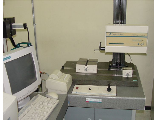
Fig. 5 Photograph of Form Talysurf Series set up for force measurement system
