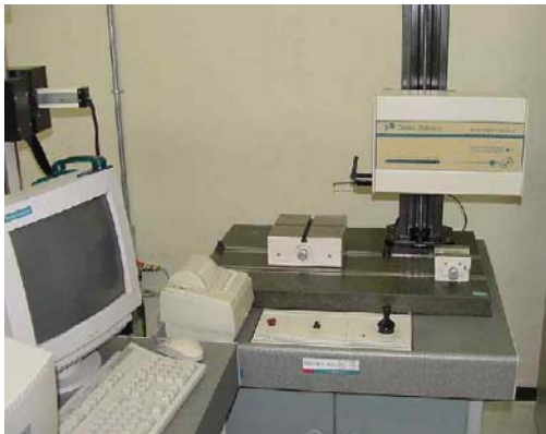
Fig. 3 Photograph of Form Talysurf Series set up for force measurement system
