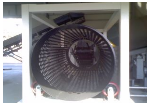
[Fig. 1] Pilot-scale reaction system for organic municipal solid waste degradation.
