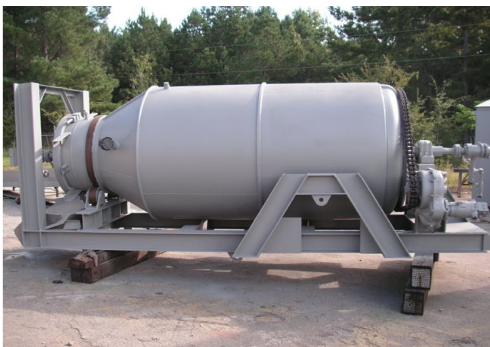
[Fig. 1] Pilot-scale reaction system for organic municipal solid waste degradation.
