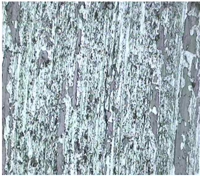
Fig. 10 Optical microstructure of tested ceramic(x200)
