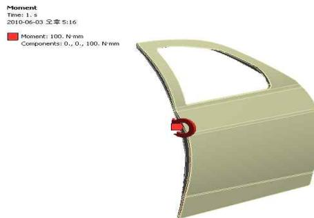
**Fig. 8 Moment condition as constraint condition at torsion**
