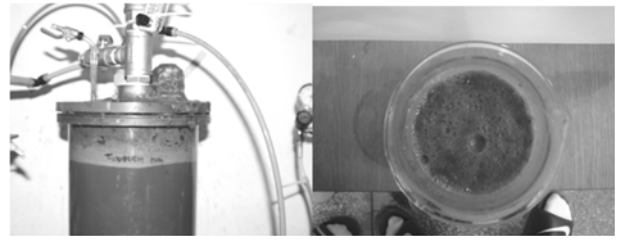
Fig. 15. Foaming trouble in the jet loop bioreactor for high organic loading.
