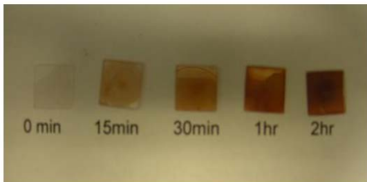
Figure 3. BaFe 12 O 19 films on sapphire(Al 2 O 3 ) substrate at various electro-spray coating times
