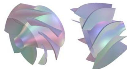
Fig. 1 3-dimensional shape of Pump-10
