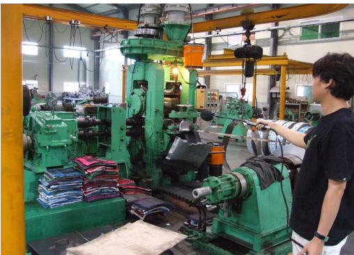
Fig. 1 Measurement of the sound power level using sound intensity probe
