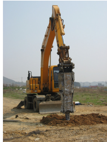
Fig. 2 A photo of noise shielded breaker
