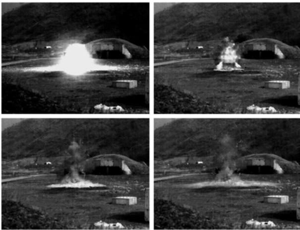
Fig. 6 Explosive scene by ANFO 15.88 kg
