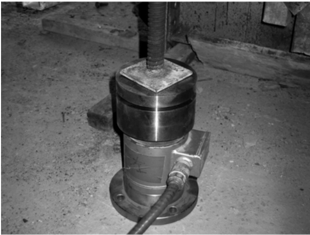
Fig. 3 Setting of load cells at the base of a shore
