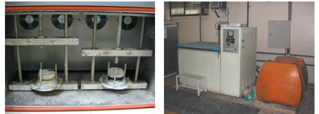
(a) Heat attack in chamber (b) Heat cycling chamber
