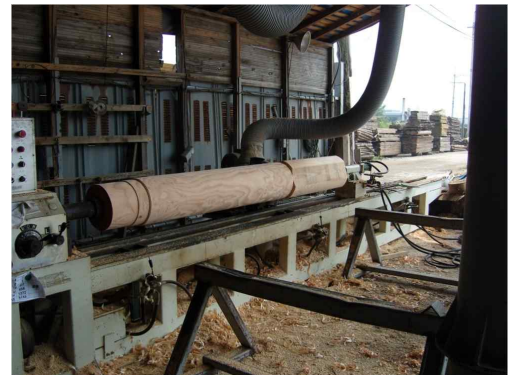
Figure 5. Member Production Automation of Han-Ok
