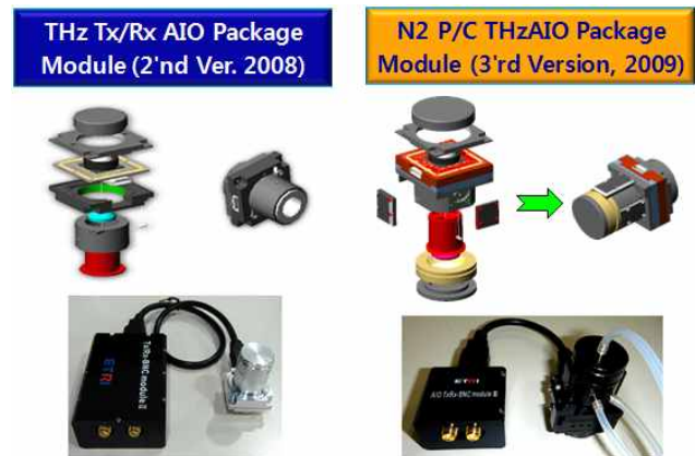
Fig. 6. THz Tx/Rx package modules of ver. 2.0 and ver. 3.0.
