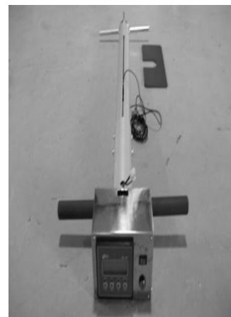
Fig. 2 The digital soil CI measuring device developed in the study.
