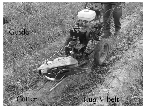
Fig. 2 The cutting device for soybeans.
