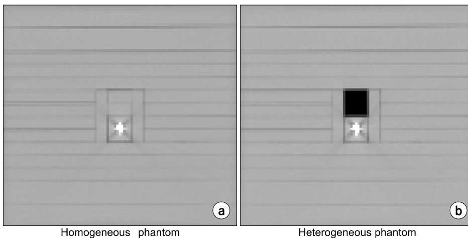
Fig. 3. The EGSPHANT formatted material and density matrices of the (a) homogeneous and (b) heterogeneous with air region phantoms. Images were derived from the DOSXYZ_show program. For both phantoms, voxel size was 2 \times 2 \times 2 \text{ mm}^3 and the dimension of the phantom was 20 (width) \times 20 (length) \times 18 (height) \text{cm}^3 .
