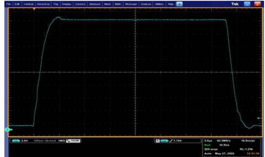
Fig. 12. The evaluation results of output slewing characteristics at 10kΩ/250pF load
