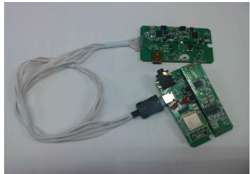
Fig. 14. Developed portable EEG measurement and wireless transmission device
