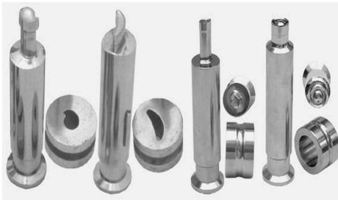
Fig. 1. The piercing tools used in the punch press.
