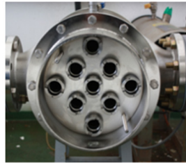
(a) Disinfection chamber
