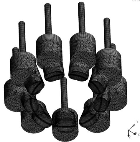
Fig. 1 Fluid models of the axial piston pumps
