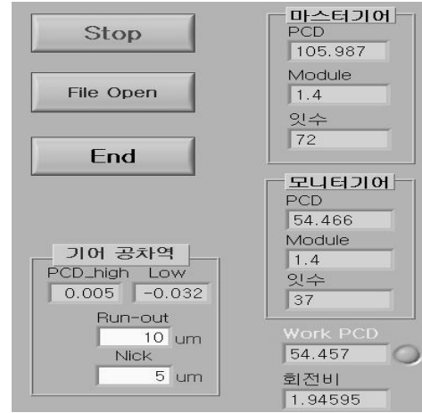
Fig. 10 An example of gear inspection software and PCD calculation window
