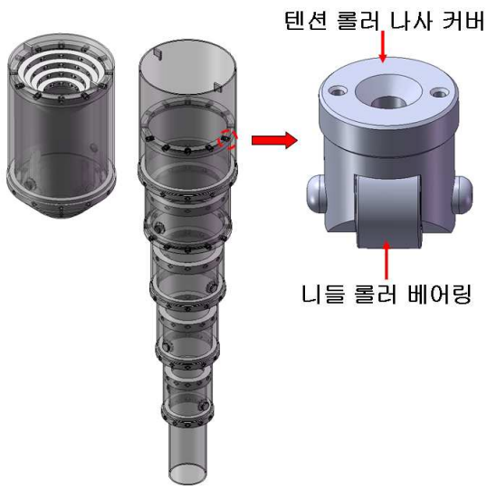
(a) Proposed telescopic tube (b) Needle roller bearings
