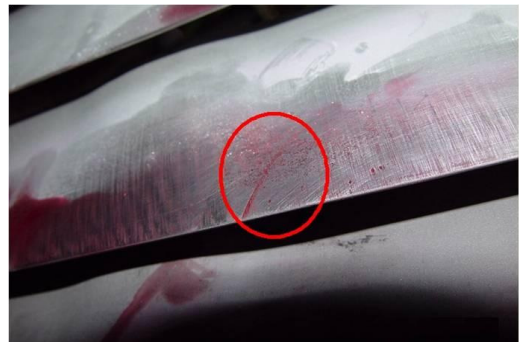
Fig. 1 Crack of a L-1 blade
