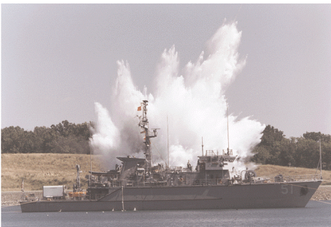
Fig. 1 Shock trial of USS OSPREY(MHC 51) at the aberdeen test center(courtesy of U.S. Navy)
