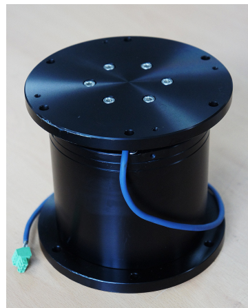
Fig. 6 Photograph of the manufactured MR damper
