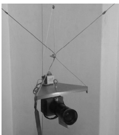
Fig. 6 The improved design using tensional object.
