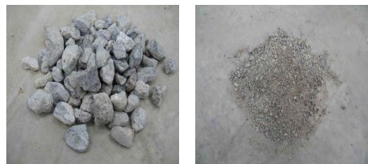
Figure 2. 순환골재 형상(25mm, 5mm)
