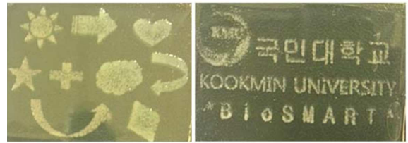
Fig. 5 Various patterns formed by colonies of bacteria deposited on the agar substrate by HP Photosmart D5360 inkjet printer.
