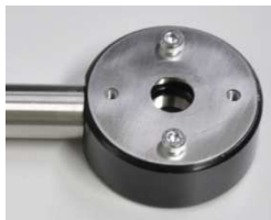
Fig. 4 Holder for confinement by BK7 glass
