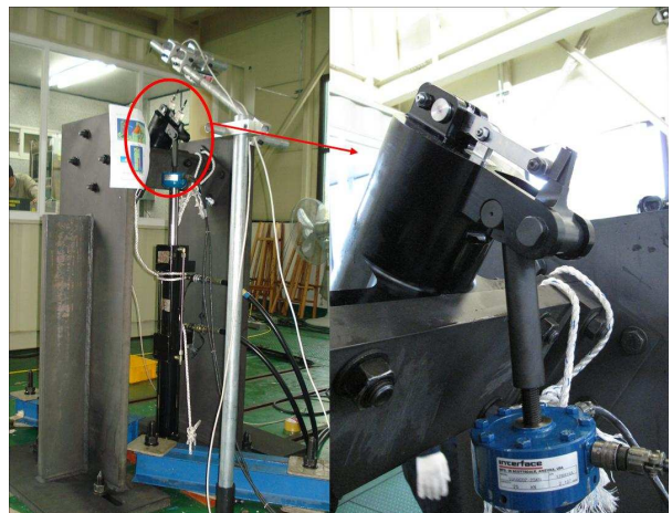
Fig. 7 Test setup for operation test of failure mechanism
