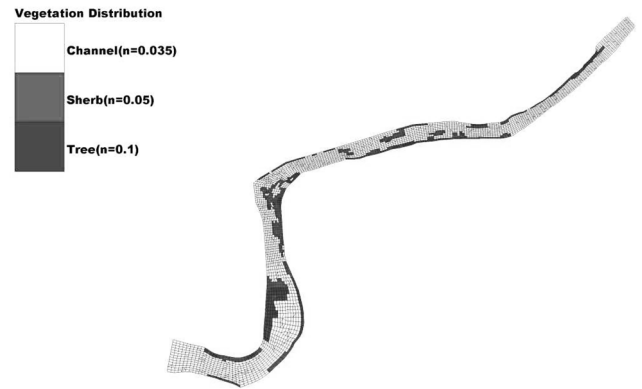
Fig. 7 Finite element mesh assigned different roughness coefficients considering vegetative distribution
