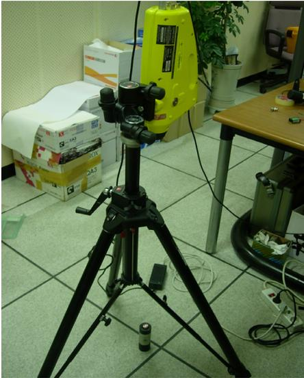
Fig. 8 Calibration experiments using calibration exciter
