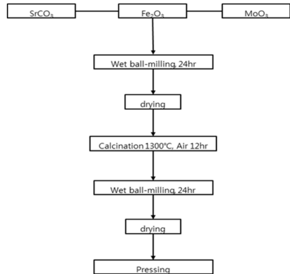
Fig. 1. Flow chart for the preparation of Sr_2FeMoO_6 powder target.
