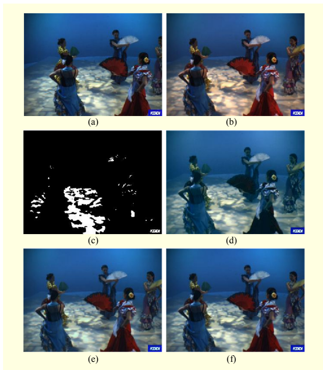
Fig. 1. Color correction results for flamenco1: (a) reference view, (b) source view, (c) highlight detection result of source view, (d) corrected view with method 1, (e) corrected view with method 2, and (f) corrected view with proposed method.
