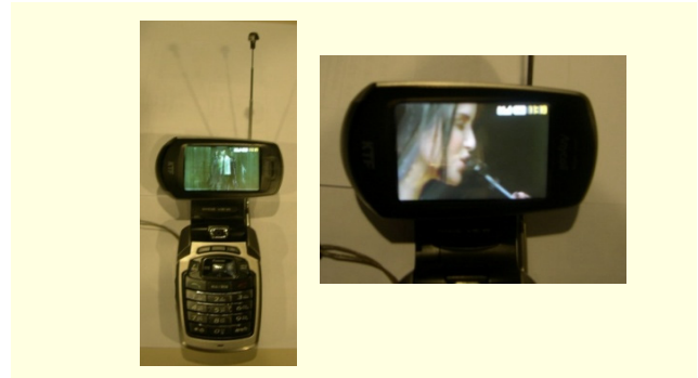
Fig. 16. Snapshot of the cell-phone-type commercial T-DMB player receiving the T-DMB multichannel audio signal.
