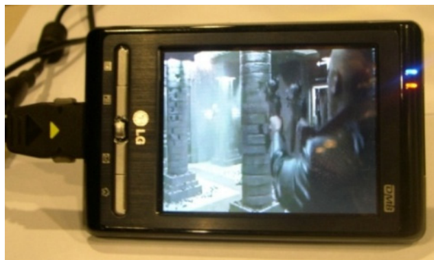
Fig. 15. Snapshot of the PDA-type commercial T-DMB player receiving the T-DMB multichannel audio signal.
