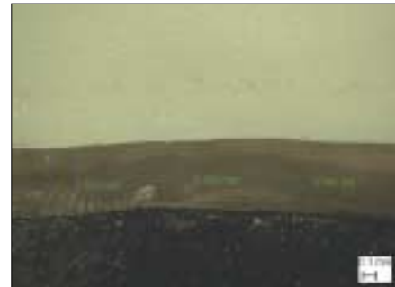
Fig. 4. Measurement of the marginal discrepancy using the video microscope system just after sintering (× 100).
