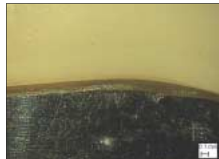
Fig. 5. Measurement of the marginal discrepancy using the video microscope system after internal adjusting and sintering (× 100).
