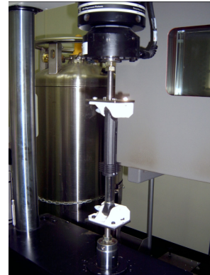
Fig. 2 Damper with a jig in testing machine
