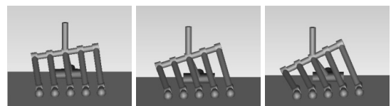
Fig. 15 Motion of the tilted foot by 10° when a weight is applied to the vertical direction (DAFUL)
