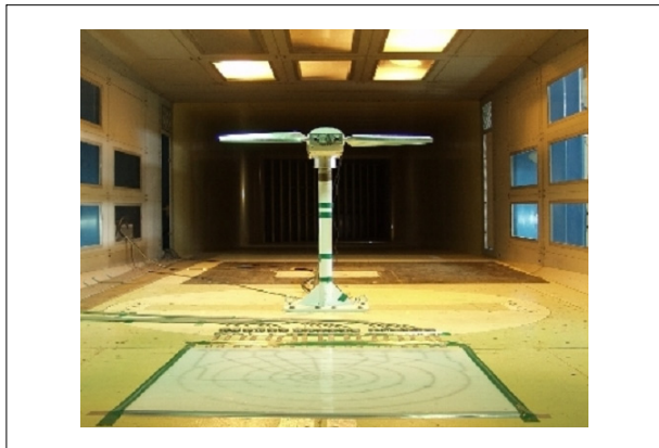
Fig. 3 Acoustc wind tunnel test for wind turbine blade
