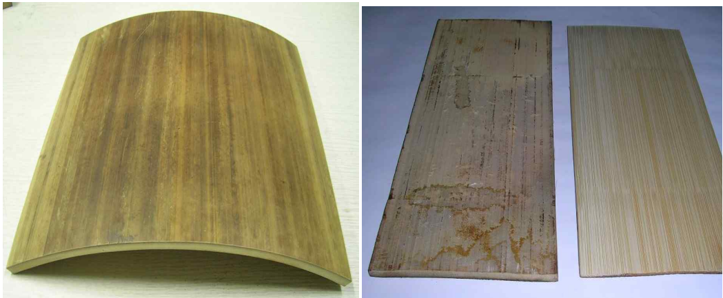
Fig. 6. Cupping of flattened bamboo(L) and planed panel(R) for re-flattening treatment.
