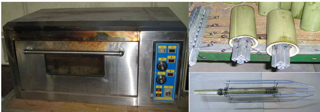
Fig. 3. Oven for preheating(L), bamboo specimens(Ru) and spring(Rl) for widening opening.
