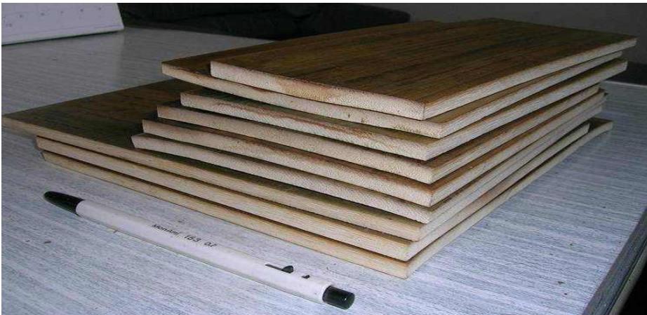
Fig. 5. Bamboo panels just after flattening treatment.
