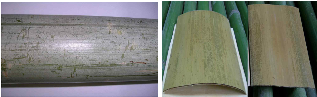
Fig. 1. Wax on bamboo skin(L) and blotted bamboo panels due to insufficient washing(M/R).
