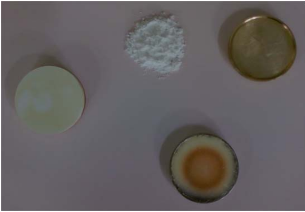
Figure 1. Photograph illustrates the sequence to produce the ZnO powder target. The sintered ceramic target typically used is also shown(left).
