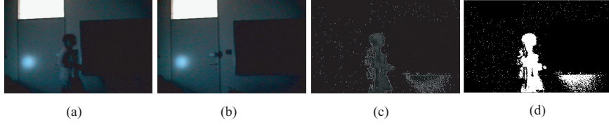
FIGURE 1. Showing the result of object detection with level set based bimodal segmentation without using regularization terms. (a) current frame (b) background frame (c) absolute difference frame (d) segmentation result (level set function).
