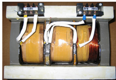
(b) Photograph of the leakage transformer
