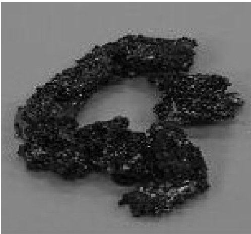
Fig. 4. Melted Fusible Metal(Y Company).
